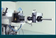
Two different kinds of second antivibration device can be installed on the lathe headstock\*\*
