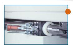
When switching from guide bushing mode to the non-guide bushing one the **Swiss & Chuck** device allows the operator to bring the bar feeder near to the lathe up to 330 mm. Because of it the installation distance is reduced and **vibrations are minimized**. The Swiss & Chuck device is extremely **simple and fast** to use even for inexperienced operators.
